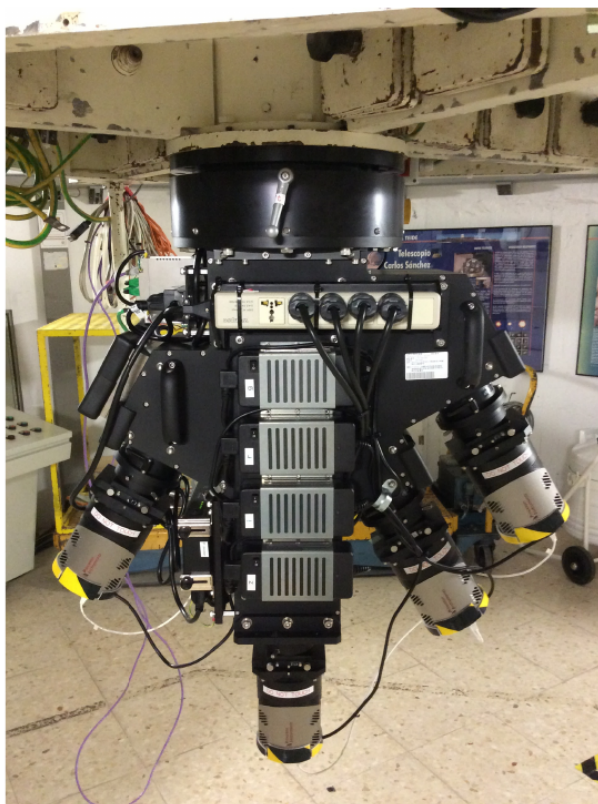
MuSCAT2 instrument mounted on TCS. The four cameras provide images obtained simultaneously with four different filters.
